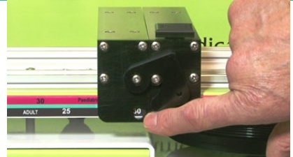
Patient pressure controlled by moving weights
