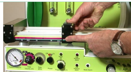
Patient pressure controlled by moving weights
